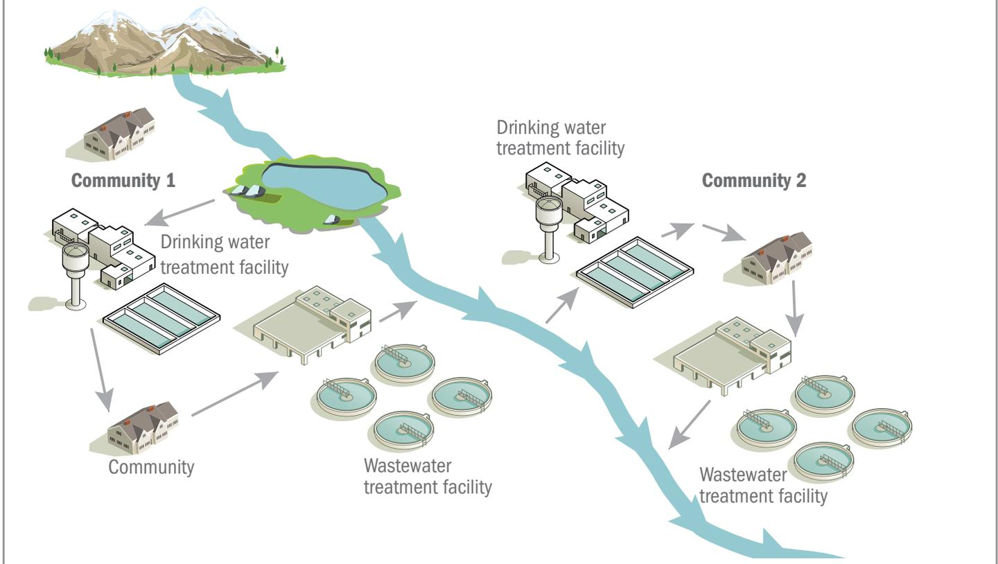
Figure 2: Flow schematic of indirect potable reuse
